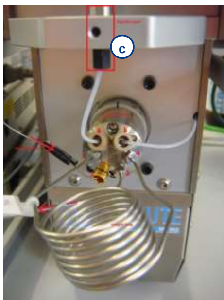
Figure 3: ThermELUTE™ module (front view)
