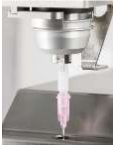
Figure 5: SMART column with needle attached taken by the SMART column gripper.
