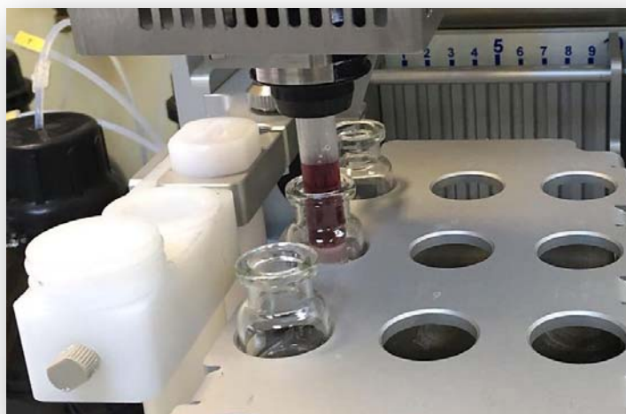
Fig. 3: BD-SPE loading step of a blood sample at the Istanbul Forensic Lab
