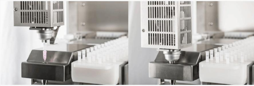
*Gripper with adapter injects SMART column into the ThermELUTE™ module.*
