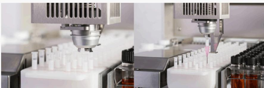
*Gripper with adapter takes the SMART column.*
