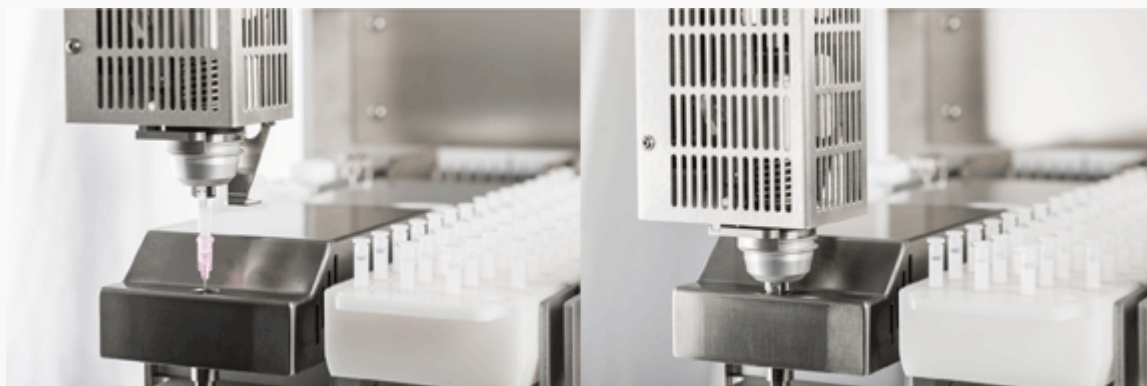
Gripper with adapter injects SMART column into the ThermELUTE™ module.
