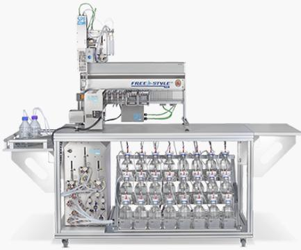
With FREESTYLE PFAS, the automated clean-up of perfluoroalkyl and polyfluoroalkyl substances from up to 24 water samples of 0.05 to 10 litres is possible fast and unattended, even at weekends and overnight.
