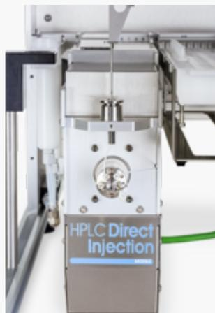
For the QuEChERS method, the FREESTYLE BASIC system is equipped with the [SPE module](#) and the [HPLC Direct Injection module](#) for the additional on-line connection to your LC-MS/MS system.
