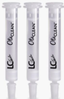
The OtaCLEAN columns are available in the practical 3 mL polypropylene format or additionally as 1 mL version. The column bed consists of a soft-gel, which is covered by a storage buffer. The storage buffer contains a preservative. The loading capacity is 200 ng ochratoxin A per column. The shelf life of the columns is 24 months at a storage temperature of 4 °C to 30 °C.
