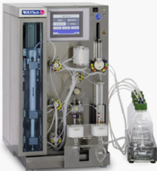
DEXTech Pure offers the unique clean-up of **PCBs and dioxins** in one “pure” fraction each. This is the perfect solution for customers interested especially in measuring PCBs and dioxins separately within one GC-MS run each or also for customers interested only in PCB analysis, as it is often relevant in the environmental sector. In this case DEXTech Pure offers a 2-column-method reducing the run time.
