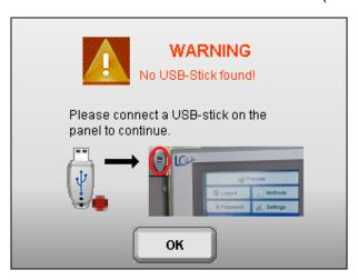
Now, a USB stick must be inserted into the device USB port (see Figure 93). Once the USB stick is connected, a report page (see Figure 95) will appear. From here, data transfer (of all previously stored sample data) can be initiated by clicking the button "to USB". All sample data stored and subsequently transferred are contained in the list.
