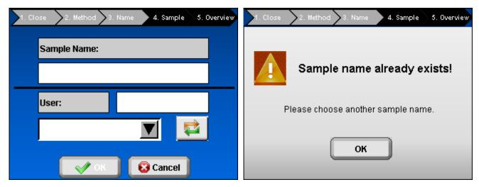
Figure 99: After input of an already existing sample name (left) a message will appear (right) prompting you to choose a different sample name.
