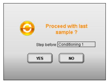
Figure 24: Display screen after power failure.
