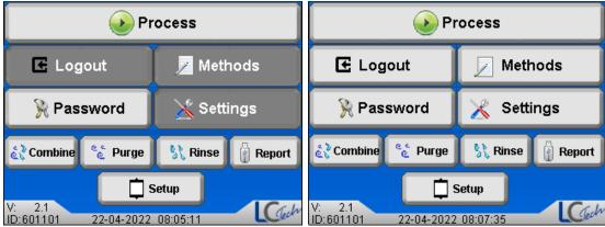
Figure 55: Left screen, locked buttons. Right screen, unlocked buttons "Create Methods" and "Settings".
