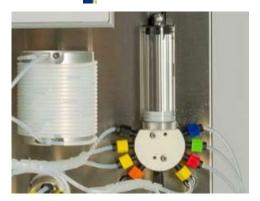
Figure 65: System components to purge sample loop.
