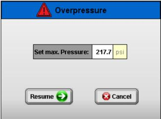
Error message 2: Overpressure fault in the system.
