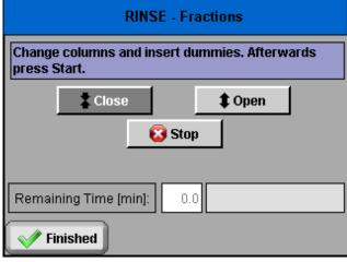
Figure 77: Left screenshot: Locked "Open" button during rinsing. Right screenshot: Finished rinsing process with the option to open the column tower.
