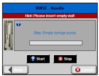
Figure 83: Emptying of the syringe pump.
