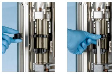
Figure 10: Handling of the SMART column. First, click the adapter into column position 1 (left) and then insert the SMART column (right).
