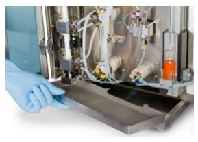
Figure 126: Removal of the drip tray.
