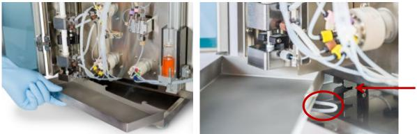
Figure 123: Left: removable drip tray; right: solvent sensor (red arrow) for solvent detection with a tube trap (circled in red).
