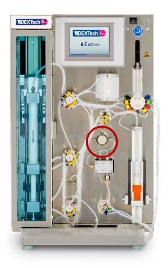
Figure 47: Calibration of the pressure sensor.
