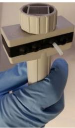
Figure 155: Preparation for flanging of the tube. Left cutting the tube end, centre assembling the materials and right insertion of the tube into the flanging holder.
