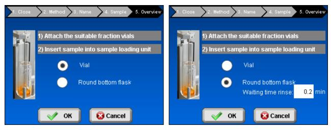
Figure 14: Reminder to provide the sample collection vials and to place the sample vial into the sample vial holder.
