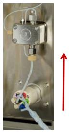
Figure 59: Purge solvent via pump.
