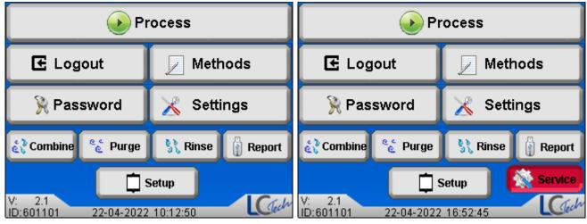
Figure 148: Main window without (left) and with (right) service display.
