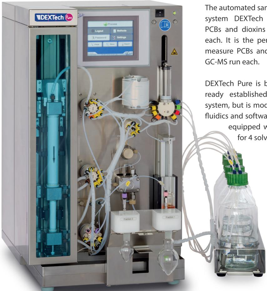
The automated sample preparation system DEXTech Pure separates PCBs and dioxins in one fraction each. It is the perfect solution to measure PCBs and dioxins in one GC-MS run each.
