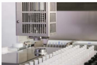
Gripper takes adapter.
